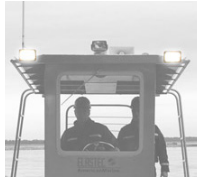
Forward Deck Flood Lamps
