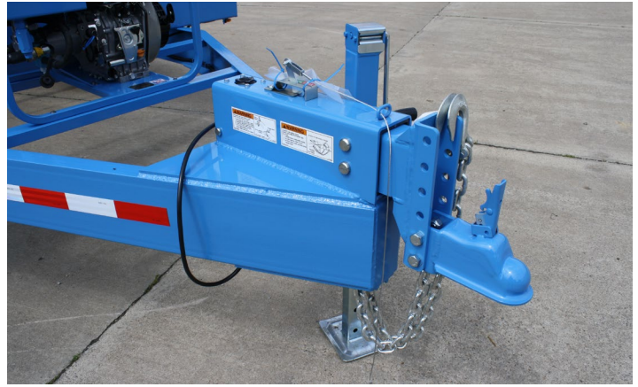
Hitch with Hydraulic Surge Brake
